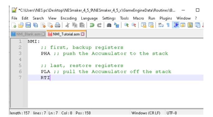
The first thing that this NMI is doing is PHA, and the last is PLA. The command PHA pushes the accumulator (PH = Push, A = the accumulator) to the stack, and PLA pulls the value off the stack and puts it back into the accumulator (PL = Pull, A = accumulator). If you're unfamiliar with this sort of programming, that sentence is a lot of words and acronyms that don't mean much. So let's put it in easier terms. We'll start with the stack.
